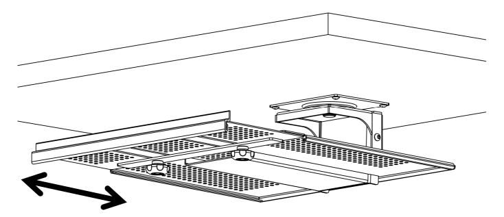
Adjust to Desire Length and Secure with Tension Knobs
