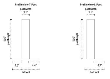
When considering space requirements, it is important to remember to include the total combination of rail and post measurements.
