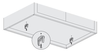
• Snap the light fixture into the mounting clips.
