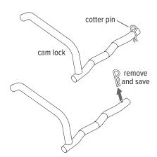
CAUTION: The cam locks must be in the locked position at all times to secure the legs in place.
