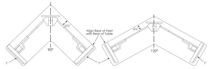
Once the frame is in its final position, attach it to the work surface using the M5x18 screws (16 total required).
