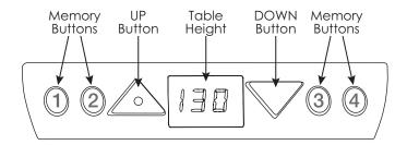
CAUTION: The "zero setting" procedure must be completed before operating the table. See Step 15 on page 9.
