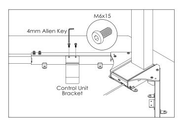
Attach the control unit to the work surface.
