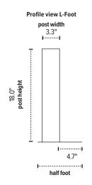
When considering space requirements, it is important to remember to include the total combination of rail and post measurements.
