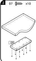
Fit slide support 05 to the underside of your computer desk ensuring it is approximately 15mm back from the front edge, and far enough away from the sides of the desk to enable the CPU to fit under the desk. Using a bradawl mark the screw positions, and secure firmly with screws 07 as shown.
