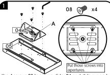
Use 4 screws 08 to secure slider 04 and slide support 05 (as figure). When securing, put those 4 screws into the apertures and use "L" allen key to tighten them.
