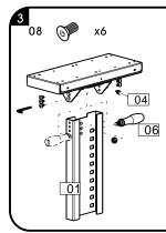
Secure the handle 06 to the top bracket 01 with nut .The handle 06 may be fitted to left or right hand side to suit left or right handed use. Secure the top bracket 01 to the slider 04 with 6 screws 08. Fully tighten with allen key provided.
