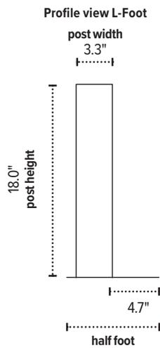
When considering space requirements, it is important to remember to include the total combination of rail and post measurements.
