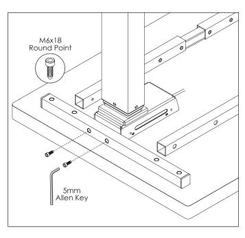
Adjust the cross channels to their approximate final lengths. • Use the 5mm Allen key to loosen the 8 set screws on the inward side of the cross channels. • Position the leg columns and top supports so that the top supports are approximately 1" (25mm) from the ends of the table. • Expand the cross channels to the top supports. • Center the inner piece in each cross channel. Loosen Set Screws Loosen 5mm Allen Key Set Screws Expand Cross Channels to Top Supports
