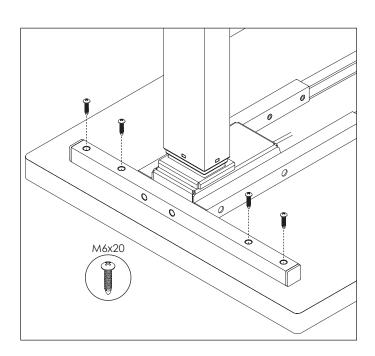
Use the 5mm Allen key to tighten the set screws (8 total) in both cross channels.
