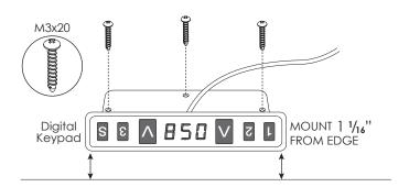
Attach the control unit using the two M5-15 Phillips round head screws.
