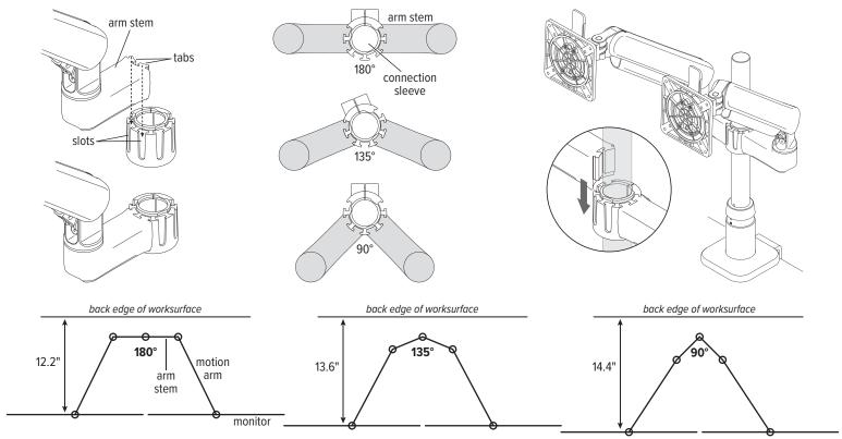
These diagrams show the approximate amount of monitor projection for different angles of the arm stems. In these examples, the units are clamp mounted at the rear of the worksurface, the motion arm is at a 30° angle to the worksurface, and the monitors are 20" wide..
